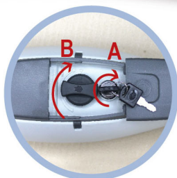
A. Turn Key 90° clockwise B. Turn release knob 180° clockwise
